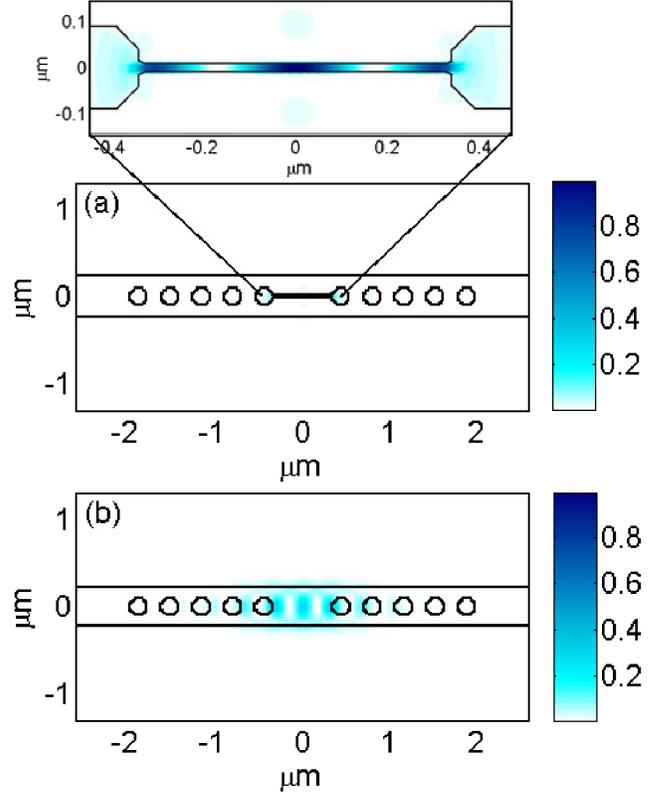
FIG. 3 (color online). (a)  $|E|^2$  field spatial distribution from 3D FDTD in the a cavity based a on buried waveguide with an embedded low index slot at its resonant wavelength of 1431.3 nm. (b)  $|E|^2$  field spatial distribution from 3D FDTD in a quasi-1D microcavity based on a buried waveguide without a slot for the resonant wavelength of 1556.4 nm.
