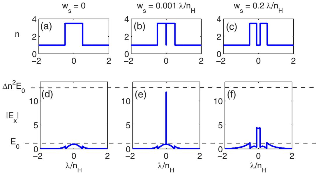
FIG. 1 (color online). (a)–(c) The index profile for the slab waveguide with embedded low index slot regions of various slot widths ( $w_s$ ). (d)–(f) The field distribution of the fundamental mode in the slab waveguide for various values of  $w_s$ . The electric field is polarized normal to the interface.  $E_0$  is the maximum value of the electric field for the slab with no slot and  $\Delta n$  is the ratio  $n_H/n_L$ .
