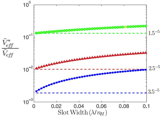
FIG. 2 (color online). The ratio of the effective mode volume of a slot waveguide compared to a slab waveguide for  $\Delta n = 1.5$  (circles),  $\Delta n = 2.5$  (triangles), and  $\Delta n = 3.5$  (squares), where  $\Delta n$  is the ratio of high to low refractive indices. The slab thickness is  $\lambda/n_H$ .
