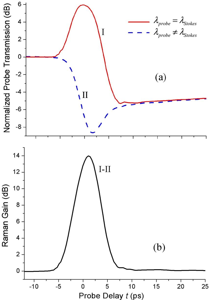
Fig. 1. (a): Normalized probe transmission versus the relative time delay between the probe and the pump when the  $\lambda_{pump} = 1589.5$  nm,  $\lambda_{probe} = 1731.5$  nm (red solid line),  $\lambda_{pump} = 1580.8$  nm,  $\lambda_{probe} = 1741.1$  nm (blue dashed line), respectively. (b): Raman gain versus the relative delay of the probe, obtained from the difference between the two lines in (a).
