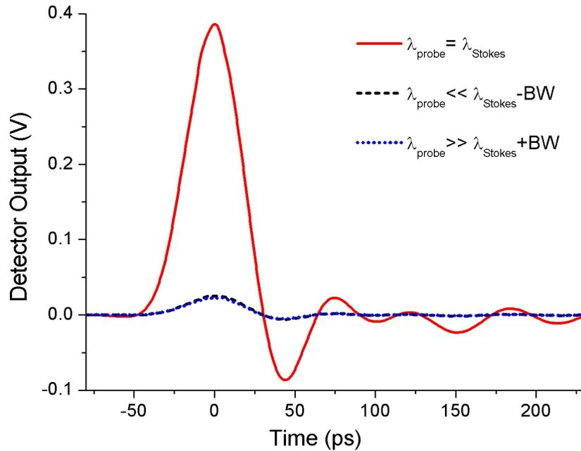
Fig. 2. The output of the ultrafast switch measured by a 12-GHz detector. Solid line:  $\lambda_{probe} = 1549.0$  nm,  $\lambda_{filter} = 1547.4$  nm. Dashed line:  $\lambda_{probe} = 1539.0$  nm,  $\lambda_{filter} = 1537.4$  nm. Dotted line:  $\lambda_{probe} = 1559.0$  nm,  $\lambda_{filter} = 1557.4$  nm. BW = 0.9 nm is the bandwidth of the Raman spectrum.
