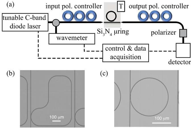
Fig. 1. (a) Schematic of the setup used for observing and characterizing polarization mode coupling in microring resonators on a temperature stabilized (T) silicon chip. (b), (c) SEM images of the microresonators and the coupling regions with the bus waveguides for (b) the 1.8 mm long microresonator and (c) a 100  $\mu\text{m}$  radius ring resonator.
