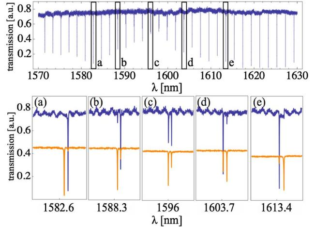
Fig. 2. Optical transmission for  $\text{TM}_{00}$  polarized light and selected resonances (a)–(e) in detail for  $\text{TM}_{00}$  (blue) and  $\text{TE}_{00}$  (orange). The appearance of the  $\text{TE}_{00}$  resonances for  $\text{TM}_{00}$  polarized input (and vice versa) and their behavior indicate an avoided crossing near 1595 nm.
