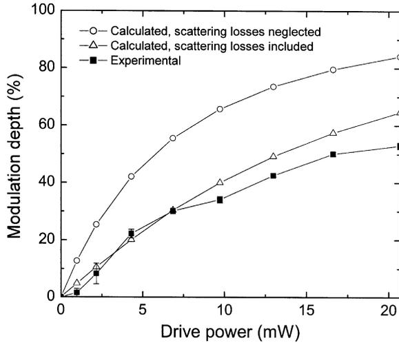
Fig. 4. Experimental (square dots) and calculated (triangular dots) modulation depth of the studied device at  $\lambda_{pb} = 1552.89$  nm as a function of the dissipated power. The calculated modulation depth of a similar device with negligible scattering losses is shown in circular dots.
