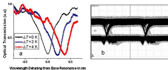
Fig. 3. (Color online) (a) Transmission spectra with varying ambient temperature with no current through the device. (b) Distorted eye diagram at  $\Delta T=2$  K, 1 Gbit/s. Applied ac-modulated voltage and wavelength of operation were unchanged.
