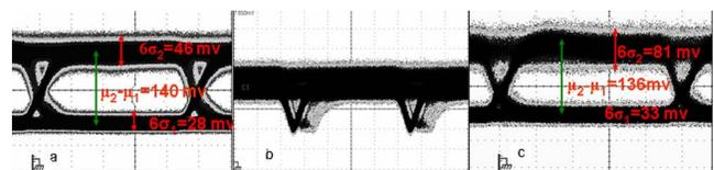
Fig. 5. (Color online) Optical transmission eye diagrams at various thermal and bias current conditions. Eye diagrams (a) at  $\Delta T=0$  K, 1.36 mA, (b) degraded at  $\Delta T=15$  K, 1.36 mA, and (c) retrieved at  $\Delta T=15$  K, 345  $\mu$ A. PRBS  $2^9-1$  bit sequences were used for all measurements. Applied ac-modulated voltage and wavelength of operation were kept constant.
