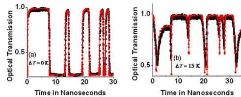
Fig. 4. (Color online) Simulation of the waveform distortion due to thermal effects. (a) Baseline simulations at  $\Delta T=0$  K. (b) Distorted waveforms at  $\Delta T=15$  K; gray curves show the electro-optic device computer simulations, and the black curves show the measured waveforms.
