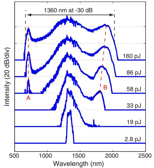
Fig. 3. (Color online) Measured spectra at the silicon nitride chip output. The spectra are progressively offset by  $20$  dB, and the pulse energy in the waveguide is indicated on the right side of each spectrum. Lines “A” and “B” highlight dispersive wave generation at short and long wavelengths, respectively.
