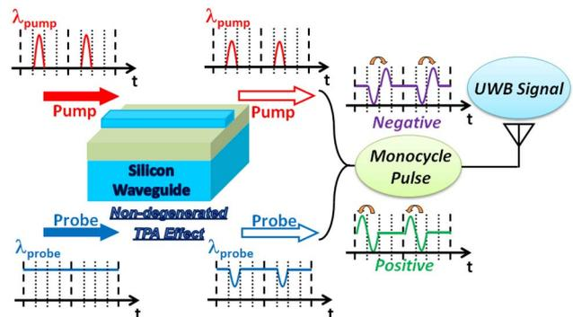
Fig. 1. (Color online) Concept diagram of silicon waveguide-based UWB monocycle pulse generation using nondegenerated two-photon absorption effect.
