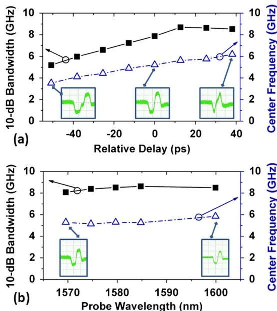
Fig. 5. (Color online) 10 dB bandwidth and center frequency of the RF spectrum as a function of (a) relative delay between the pump and inversely modulated probe ( $\text{FWHM}_{\text{pump}} = 68$  ps); (b) probe wavelength ( $\text{FWHM}_{\text{pump}} = 68$  ps,  $\lambda_{\text{pump}} = 1550.4$  nm).
