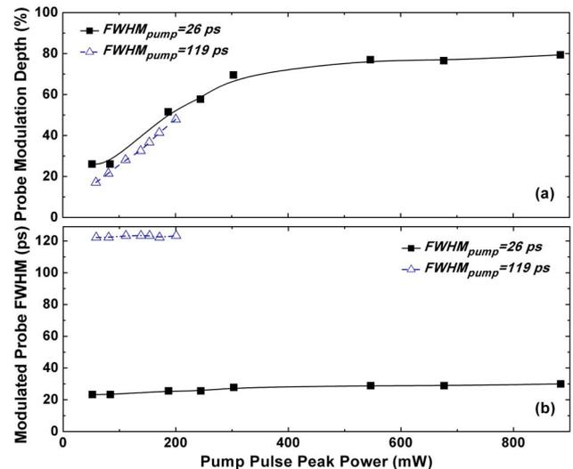
Fig. 3. (Color online) Effects of nondegenerated two-photon absorption. (a) Probe modulation depth, and (b) modulated probe FWHM as a function of pump pulse peak power for different pump pulse width.
