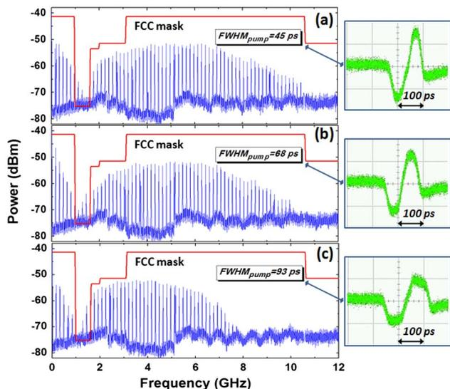
Fig. 4. (Color online) Ultrawideband signal generation. RF power spectra of generated monocycle pulse with (a)  $\text{FWHM}_{\text{pump}} = 45$  ps, (b) 68 ps, and (c) 93 ps.
