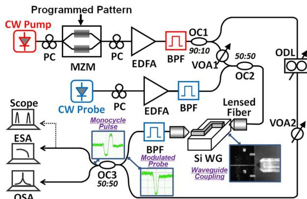
Fig. 2. (Color online) Experimental setup. Pulsed pump and CW probe are coupled to Si WG. The inversely modulated probe then combines with the pump to generate monocycle pulses.
