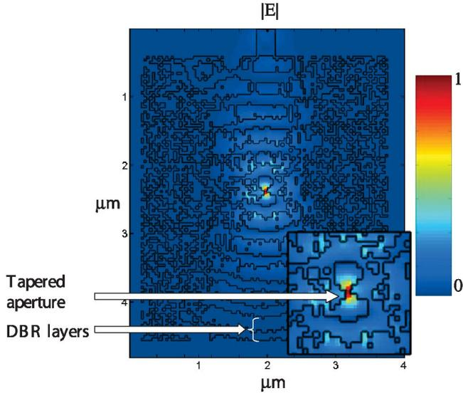
FIG. 2 (color). Normalized field amplitude of optical mode in an evolved resonator (5000th generation). The inset shows that most of the field is localized in the center slot.
