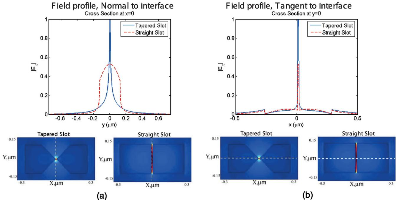
FIG. 3 (color). Propagation eigenmodes. (a) Field localization, normal to the interface. (b) Field localization, tangent to the interface.
