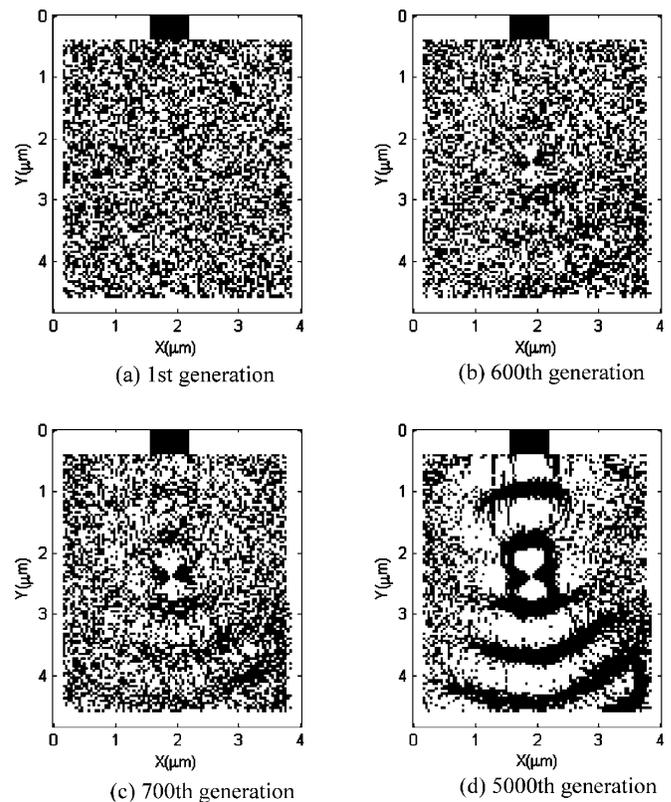
FIG. 1. Evolution of resonator (black: high index, white: low index). (a) Random starting region, (b) disturbed Bragg reflector (DBR) layers begin to form, (c) DBR layers begin to emerge, (d) DBR layers are clearly defined.
