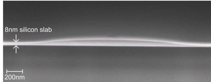
Fig. 3. Cross-section SEM image of an etchless waveguide.
