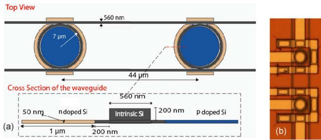
Fig. 2. (Color online) (a) Schematic of an electro-optically integrated double ring-cavity. (b) Microscope image of the device.
