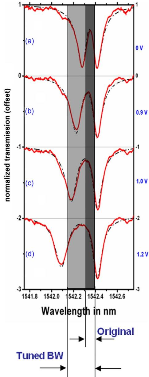
Fig. 3. (Color online) Experimental transmission spectra (solid curve) and theoretical fits (dashed curves). The curves correspond to transmission spectra as the applied voltage to one of the resonators is varied from 0 to 1.2 V. The transmission spectra (b)–(d) are vertically offset for clarity.
