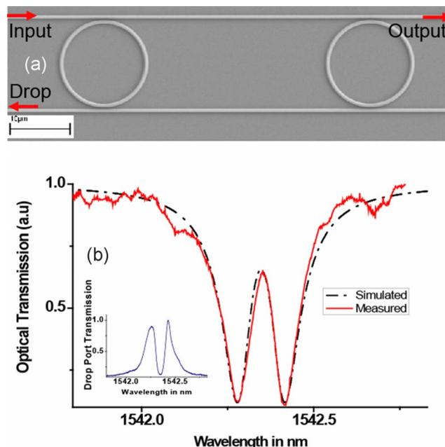
Fig. 1. (Color online) (a) SEM image of double-ring cavity. (b) Transmission spectrum of the device (the drop port spectrum is shown in the inset).
