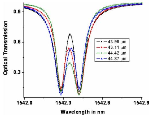
Fig. 4. (Color online) Sensitivity of the supermode transmission to changes in the distance between the coupled cavities. A 1% change in the distance between the cavities shows a 30% change in the transmission of the supermode.
