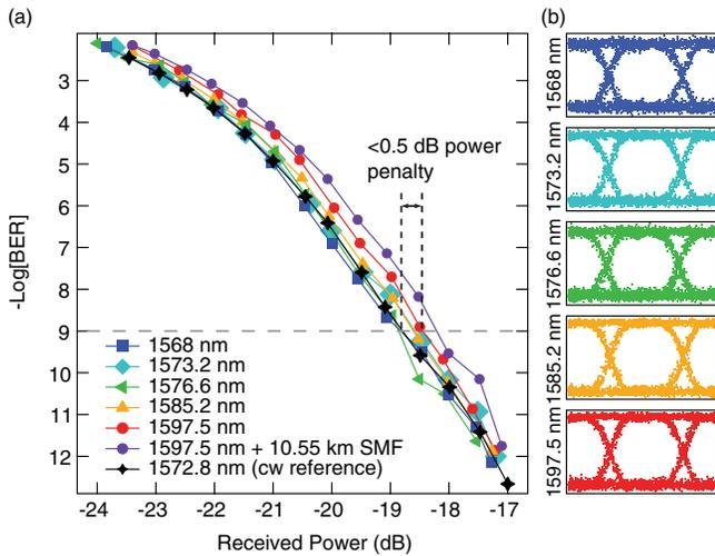
Fig. 3. (a) BERT measurements of the filtered comb lines. The cw reference measurement acts as a back-to-back baseline with which to compare the modulated comb lines. We note error-free operation of the comb lines and a minimal power penalty measured at a bit-error-rate of  $10^{-9}$ . (b) Eye diagrams for the five measured comb lines generated by the microcavity for 1568 nm, 1573.2 nm, 1576.6 nm, 1585.2 nm, and 1597.5 nm. The clean and open eye confirms the BER data showing no power-penalty.
