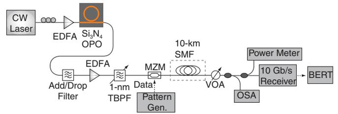
Fig. 2. Experimental setup for frequency comb generation and BER measurement. The comb output is filtered and modulated for bit-error rate (BER) measurements. MZM: Mach–Zehnder modulator. TBPB: tunable band-pass filter.
