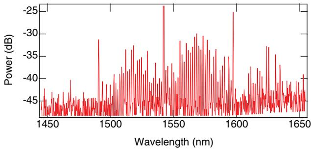
Fig. 1. Optical spectrum of the generated frequency comb at the output of the  $\text{Si}_3\text{N}_4$  waveguide with a pump wavelength of 1541 nm. The comb is in a stable low-noise state with this spectrum and we are able to manipulate and process the generated frequencies when filtering out the pump.
