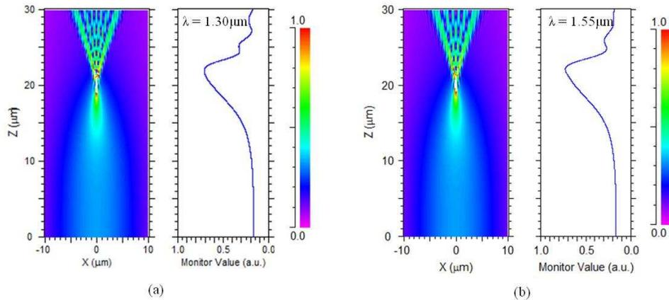
Fig. 3. Amplitude of the field for lens with dimensions 20  $\mu\text{m}$  x 20  $\mu\text{m}$ , and with homogeneous index distribution (as in Fig. 2(a)): (a)  $\lambda = 1.30 \mu\text{m}$ , (b)  $\lambda = 1.55 \mu\text{m}$ .
