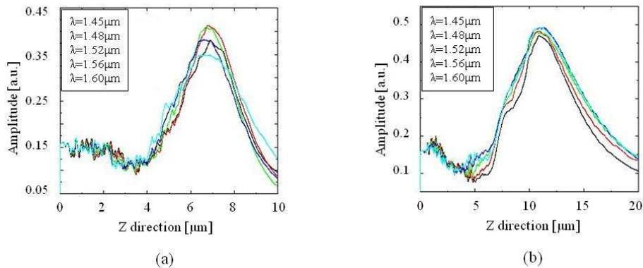
Fig. 5. Power intensity distribution for a lens with discrete index refraction and focal spot equal to 35% of the width. Lens dimension: (a)  $5\ \mu\text{m} \times 5\ \mu\text{m}$ , (b)  $10\ \mu\text{m} \times 10\ \mu\text{m}$ .
