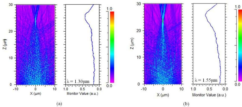
Fig. 4. Amplitude of the field for lens with dimensions  $20\ \mu\text{m} \times 20\ \mu\text{m}$ , and with discrete index distribution (as shown in Fig. 2(b)): (a)  $\lambda = 1.30\ \mu\text{m}$ , (b)  $\lambda = 1.55\ \mu\text{m}$ .
