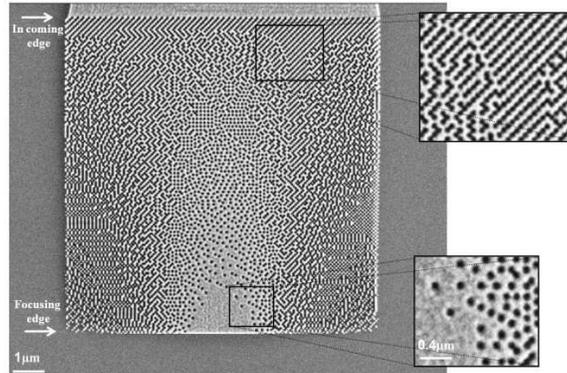
Fig. 6. Scanning electron microscope of a fabricated lens with dimension  $10\ \mu\text{m}$  x  $10\ \mu\text{m}$ . 80nm air-holes are etched in SOI wafer with varying density determine the distribution of the effective index of the lens. The distribution of the air holes is given by the design shown in Fig. 2(b). Also shown are SEMs of the incoming edge area and in the focusing edge area.
