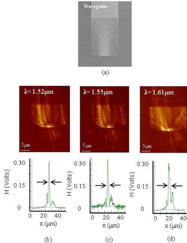
Fig. 7. (a) SEM of the lens; NSOM images for  $20\ \mu\text{m} \times 20\ \mu\text{m}$  lens dimension,  $\text{FS} = 7\ \mu\text{m}$ , for three different input wavelengths: (b)  $\lambda = 1.52\ \mu\text{m}$  (c)  $\lambda = 1.55\ \mu\text{m}$  (d)  $\lambda = 1.61\ \mu\text{m}$ . The plots in green represent the power intensity measured at the output of the sample.
