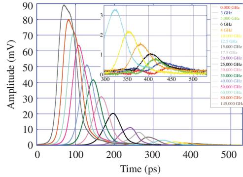
Fig. 3. Wideband optical pulse from TTD device for different detuning values from 0 to 145 GHz; inset shows zoom-in on low detuning values.
