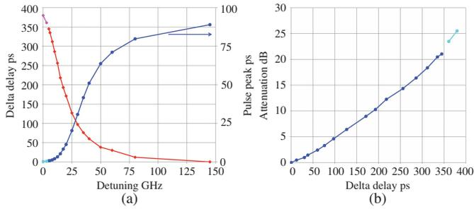
Fig. 4. (a) Plot of delay and pulse amplitude versus detuning frequency. (b) Attenuation (dB) versus delta delay.
