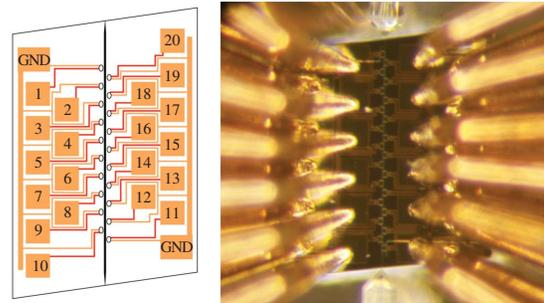
Fig. 1. Schematic and photograph of true time delay device.
