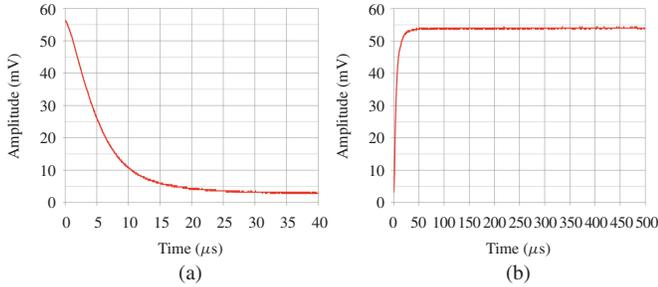
Fig. 5. Switching transients. (a) 10GHz–50GHz. (b) 50GHz–10GHz detuning.
