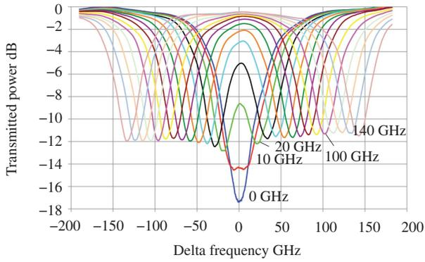
Fig. 2. Measured transmission spectra of Balanced SCISSOR versus detuning.
