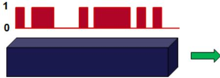
Figure 7: Bandwidth density: The bandwidth density of the waveguide is given by the aggregate data rate in the waveguide divided by the separation of two consecutive waveguides in an array of waveguides.
