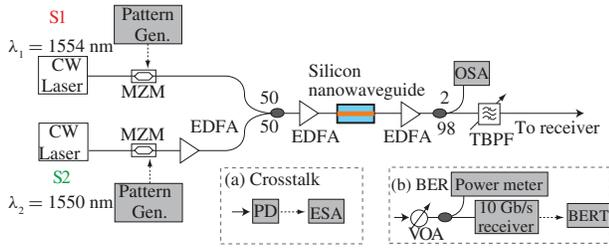
Fig. 1. Experimental setup for crosstalk measurements for a silicon nanowaveguide. Signals S1 and S2 are combined and coupled into the nanowaveguide. The output is filtered and sent to (a) for crosstalk measurements using an electrical spectrum analyzer (ESA) and (b) for bit-error rate (BER) measurements. MZM, Mach-Zehnder modulator; TBPF, tunable bandpass filter.
