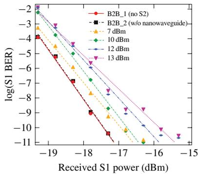
Fig. 4. Experimental measurement of the BER for various S2 powers. The numbers represent the power inside the nanowaveguide and S1 and S2 have equal powers. Two B2B measurements are performed, one without S2 and the other without the nanowaveguide.
