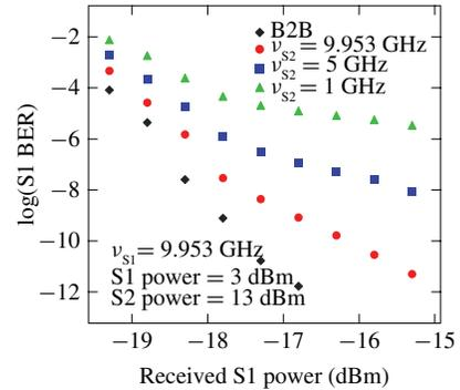
Fig. 3. Experimental measurements of bit error rate (BER) for S1 through the nanowaveguide for S2 modulation frequencies of 1, 5, and 9.953 GHz, and a back-to-back (B2B) measurement without the nanowaveguide (diamond).
