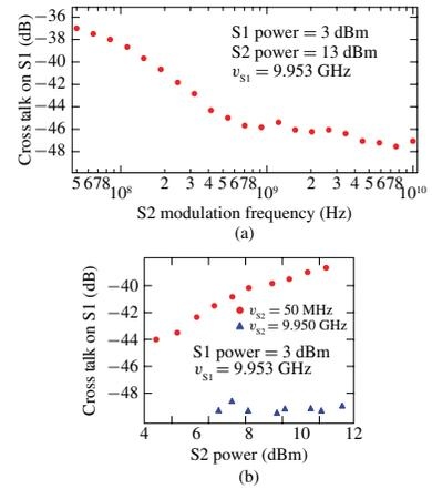
Fig. 2. Experimental results. (a) Crosstalk as a function of S2 modulation frequency. (b) Crosstalk as a function of S2 power for S2 modulation frequencies of 50 MHz and 9.95 GHz. The S1 modulation frequency is fixed at 9.953 GHz.
