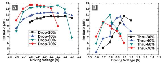
Fig. 4. Extinction ratio of the gating signal with variable driving voltages and duty cycles (30%, 40%, 60%, and 70%) for the (a) drop port and (b) through port. The waveform utilizes a 1536-ns period.
