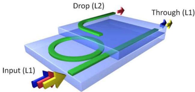
Fig. 3. 3-D integration of SiN waveguides coupled by ring resonator.
