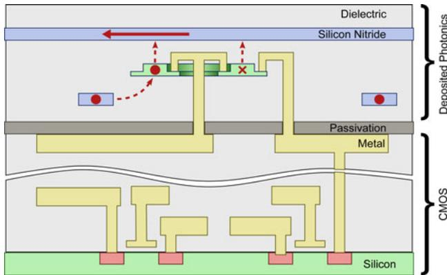
Fig. 1. Cross-sectional view of BDSP. The boundary between traditional CMOS and deposited photonics is clearly delineated.
