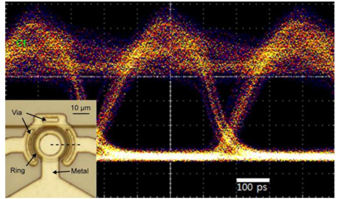
Fig. 2. Optical eye diagram of deposited polysilicon modulator for nonreturn zero 2.5 Gb/s 27-1 pseudorandom binary sequence signal.
