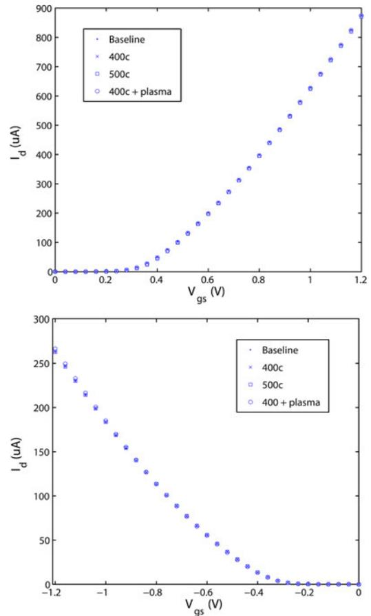
Fig. 4.  $I$ - $V$  curves of drain current versus gate voltage of transistors after going through various processing conditions (Top) N-type transistors. (Bottom) P-type transistors.
