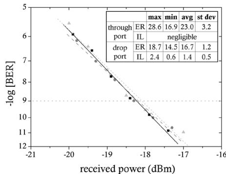
Fig. 3. BER curves taken for a signal consisting of 1 ( $\blacktriangle$ ), 12 ( $\bullet$ ), and 16 ( $\blacksquare$ ) channels passively exiting the drop port of the switch. The measurements are taken on channel C36 with a peak injection power of  $-6$  dBm. The inset shows statistics relating to the passive ERs and ILs through both switch ports (obtained from data shown in Fig. 2).
