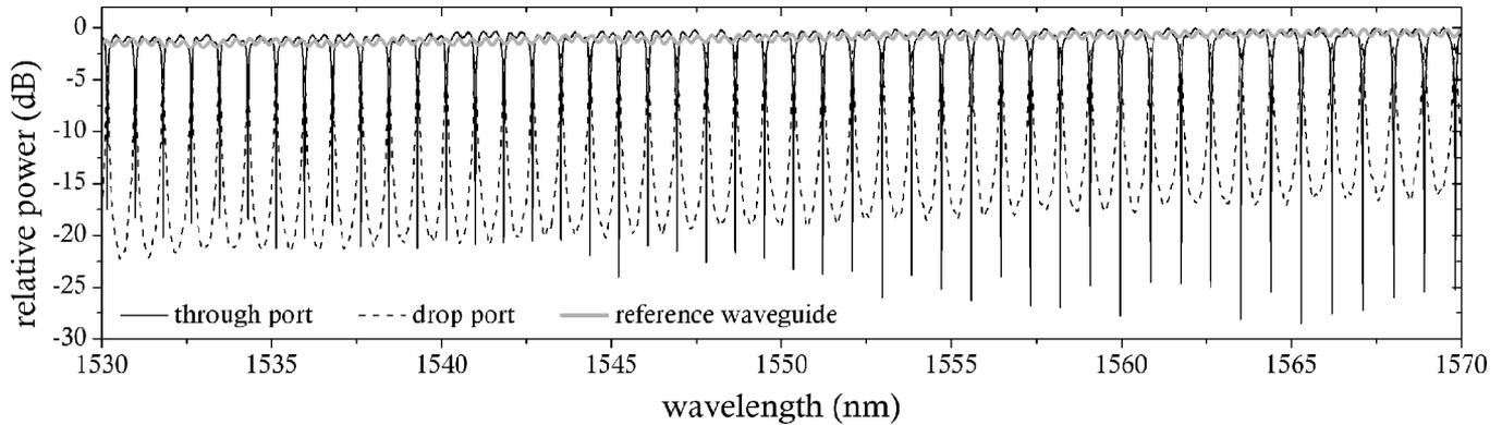
Fig. 2. Relative transmission spectrum over the *C*-band of the through port (black, solid), drop port (black, dashed), and output of the reference waveguide (gray, solid), which is used to evaluate the through port IL. See Fig. 1 for output port definitions.
