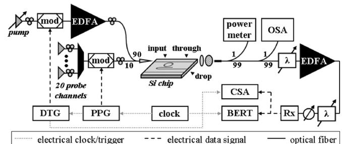
Fig. 1. Diagram of the device structure and experimental setup used for active measurements. (CSA: communications signal analyzer; DTG: data timing generator;  $\lambda$ : tunable grating filter; mod: 10-Gb/s LiNbO<sub>3</sub> modulator; OSA: optical spectrum analyzer; Rx: receiver).
