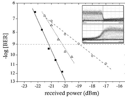
Fig. 4. BER curves recorded for a single channel exiting the through ( $\Delta$ ) and drop ( $\circ$ ) ports actively, and back-to-back measurements through a reference waveguide with no pump ( $\blacksquare$ ). The inset traces are from the drop port with no averaging, 2-ns/div time scales, and no limiting amplifier in use.
